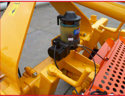
Automatic grease system for rotating bar bearings
