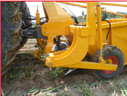
Hydraulic driven 2nd web in combination with webstop
