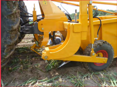
Automatic depth control in combination with driven discs
