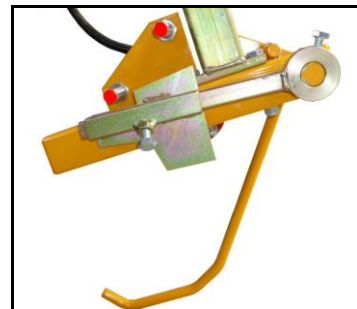
Position of reaction arm with plate relative to the sensors.
