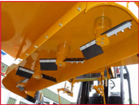
Knives in a topper with side delivery
